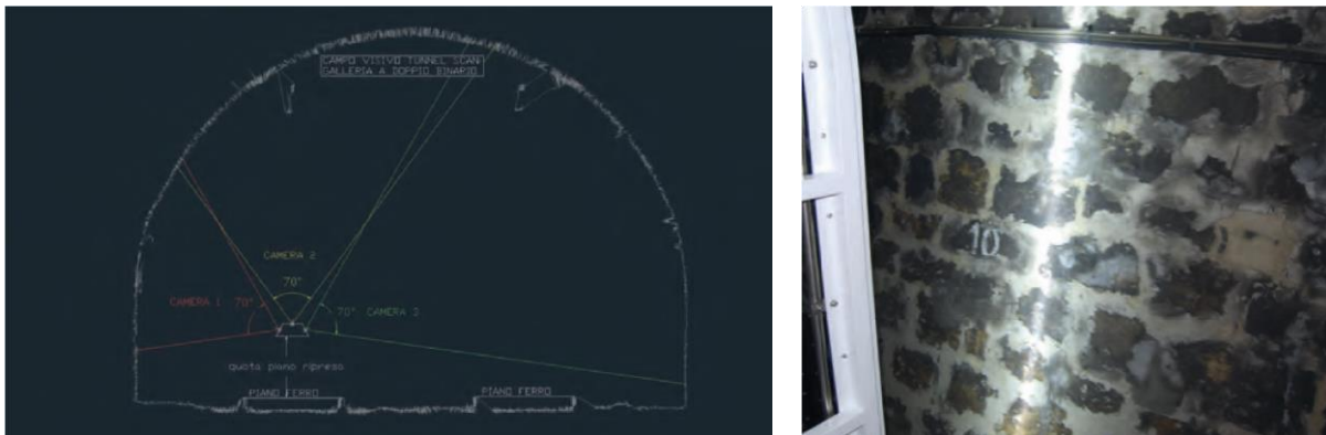
Figure 1. ARCHITA photographic scanning: field of view (on the left) and light detail during an acquisition along the line (on the right)
